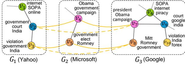
Figure 5. An example of simply adding constraints to pairwise matching. The matching result of  $f_{G_1 G_3}$  is regarded as the constraint of pairwise matching  $f_{G_1 G_2}$  and  $f_{G_2 G_3}$ . There is no correspondence between  $v_1$  and  $v_6$  because they do not have a related node in  $G_2$ .
