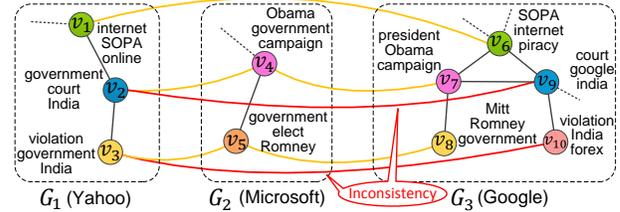
Figure 4. Inconsistency caused by directly applying pairwise matching to multi-graph matching. The node mappings between  $G_1$  and  $G_3$  derived from the matching results of  $f_{G_1 G_2}$  and  $f_{G_2 G_3}$ ,  $v_2 \mapsto v_4$  and  $v_4 \mapsto v_7$ , are inconsistent with the direct matching result of  $f_{G_1 G_3}$ ,  $v_2 \mapsto v_9$ . Here  $v_i \mapsto v_j$  indicates that  $v_i$  is mapped to  $v_j$ .
